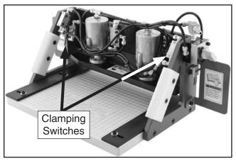
**Figure 17.** Clamping the workpiece.
